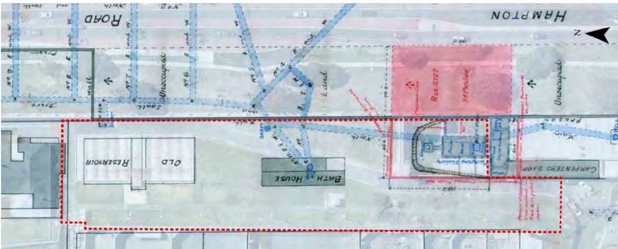
Figure 13. The 1899 sewerage and drainage plan indicates the locations of plumbing to the east and south of the Bath House, as well as earliest plan of the Engine House. This plan shows the horseshoe shaped landform created around the north side of the Engine House, indicating excavation to construct the Engine House, and the probable destruction of archaeology in this location as a result.
