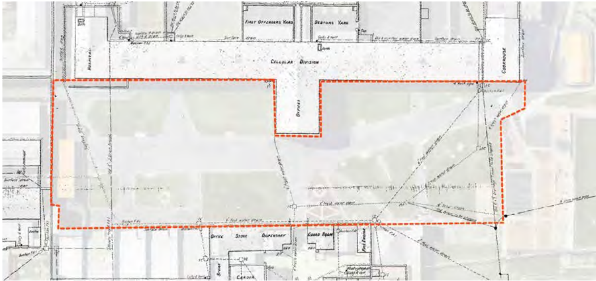
Figure 82. In the 1899 plan both the convict era tunnel drains are still visible. The location of the previously recorded mains services in the northern section of the zone is now labelled as a 'surface drain'. Details of fresh and foul water drains in the western and southern parts of the zone are shown, as well as the location of an 'old drain to be stopped'.
