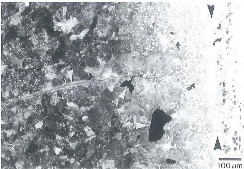
FIG. 10. Microstructure of the crown region (identified by an arrow in Fig. 3) of the insert in the unused axe. The crack and cavities indicated by the white arrows are the result of partial grain boundary liquation during welding. The weld line is indicated by the black arrows. Light micrograph; etched in 2% nital.
