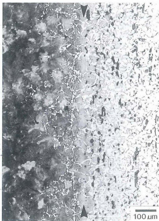
FIG. 8. Section of the forge weld between the wrought iron (right) and the steel insert (left) at the bit of the unused axe. The weld line is indicated by the light-etching band (arrows). Good bonding was achieved along the weld and diffusion of carbon occurred across the weld plane from the steel into the wrought iron. Note that the inclusions in the wrought iron adjacent to the weld are much smaller than those remote from the weld [cf. Fig. 3(b)] because the original inclusions were fragmented by the strains imposed during welding. Light micrograph; etched in 2% nital.
