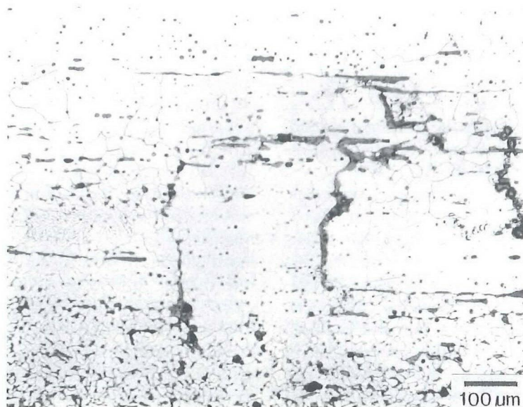
FIG. 11. Microstructure of a region in the wrought iron blade of the unused axe adjacent to the weld to the bit insert and close to the area at which partial liquation had occurred in the insert. Nonmetallic inclusions in the wrought iron appear to have melted and penetrated along the austenitic grain boundaries that existed in the iron at the time. Light micrograph, etched in 2% nital.
