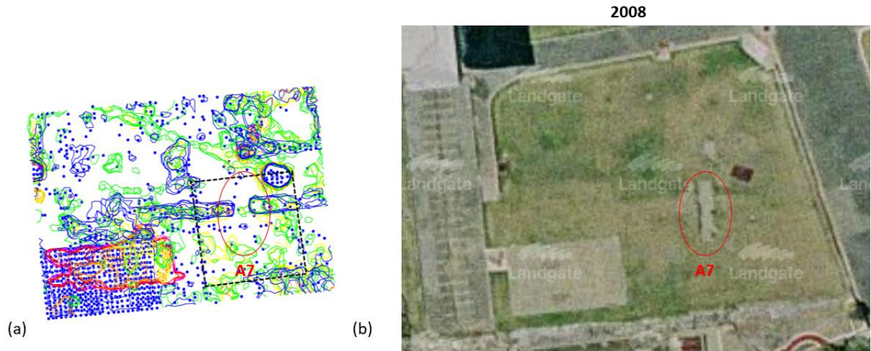
Figure 14. Common feature highlighted (red outline) between (a) GPR interpretation (showing area estimated to contain the historical well of interest (black dashed line)) and (b) historical satellite image (circa. 2008) (satellite image source: Landgate Imagery Online).
